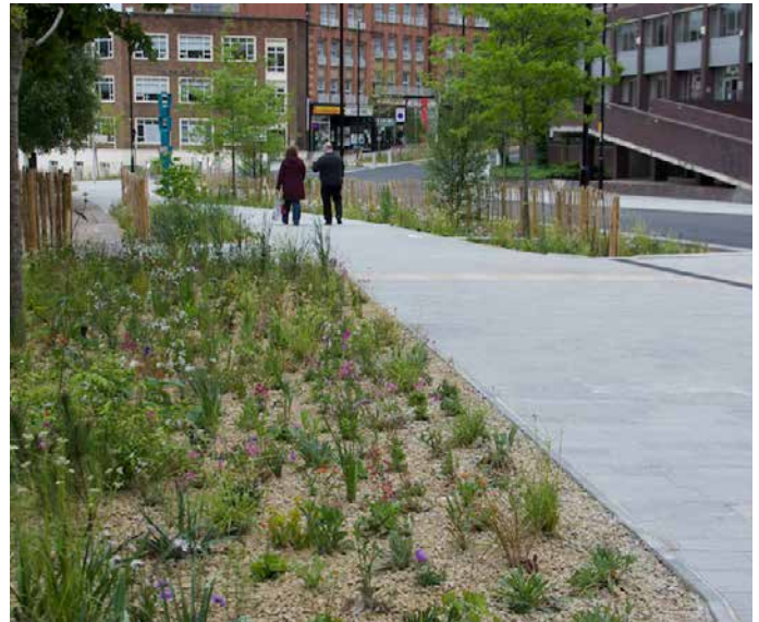
Planting in Sheffield using a substrate containing crushed quarry waste, sand and recycled compost
